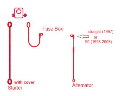
Important: Thick wire goes to engine block.
